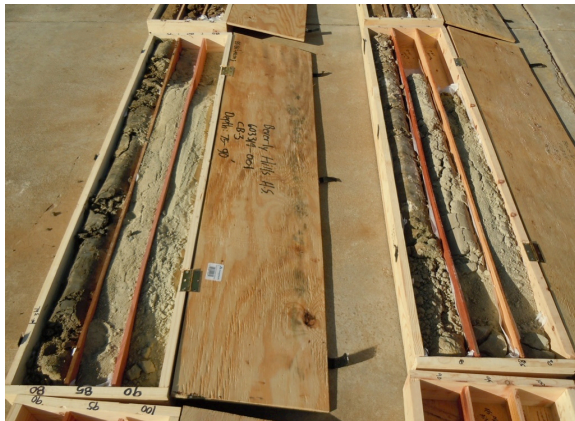
Fig. 5: Borehole correlations were made across all of the borings on the two transects to look for vertical separations of key marker units that might confirm the faults shown by Metro. Here, there is excellent correlation of the underlying San Pedro contact between borings CB-3 (left) and CB-4 (right) at ~25-30 m, despite being on opposite sides of a mapped fault.
